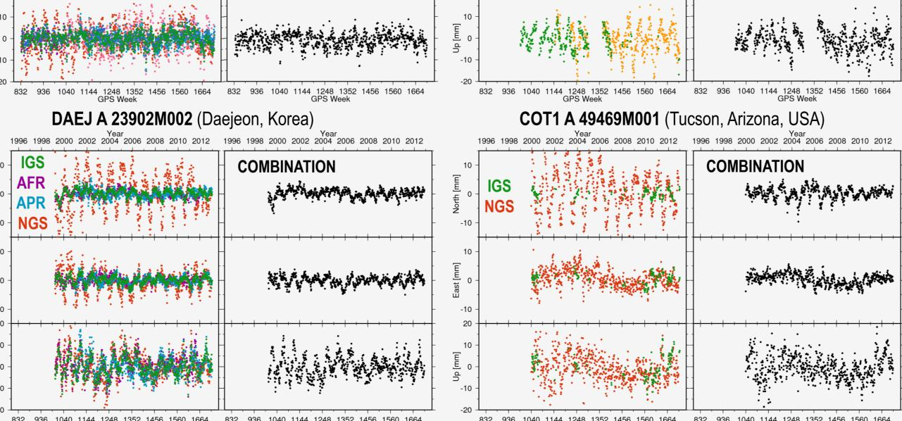
Figure 5: Residual position time series with respect to cumulative solution of individual weekly regional solutions (left) and weekly combined solution (right).
