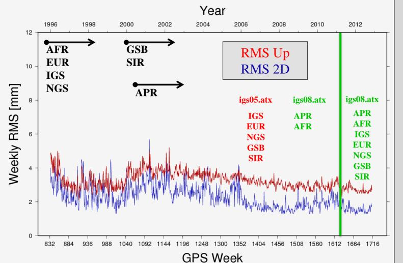
Figure 2: RMS [in mm] of the weekly combinations as a function of time (Up in red and 2D horizontal in blue)
