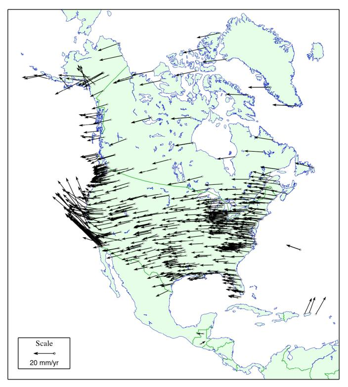
Figure 4: Horizontal velocities from NAREF cumulative solution.
