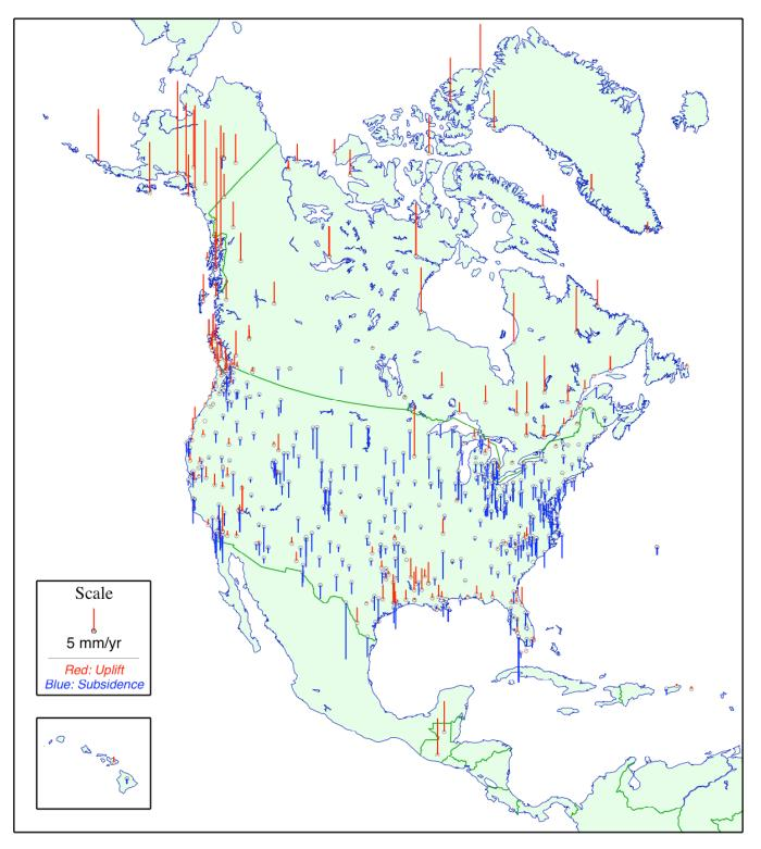
Figure 6: Vertical velocities from NAREF cumulative solution.
