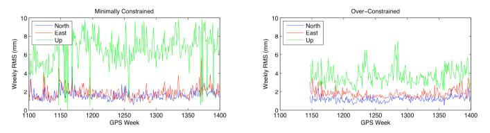
Figure 3: RMS of NAREF weekly solutions with respect to IGS weekly combinations.
