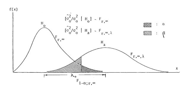
Figure 3.2 Probability distribution function of test statistic y under  $H_0$  and  $H_1$  (after Kavouras [1982]).
