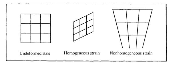
Figure 4.1 Examples of homogeneous and nonhomogeneous deformations.
