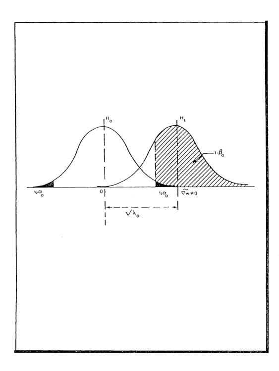
Figure 3.3  $\sqrt{\lambda_0}$  shows the shift of the standard normal distribution of w when H<sub>1</sub> is true (after Kok [1984]).
