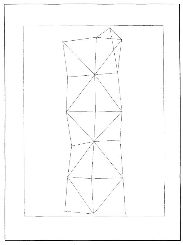
Figure 7.2 Direction observations for simulated 3D HOACS network.
