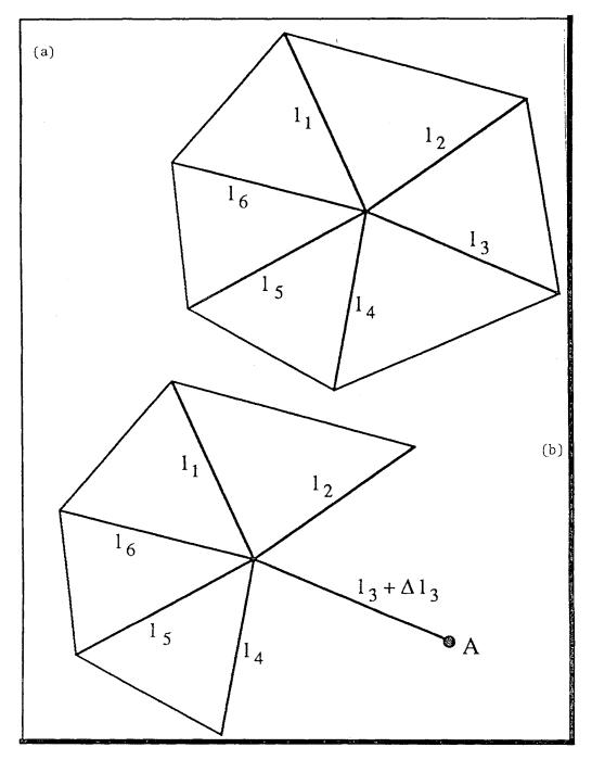
Figure 2.1. Detectability of blunders and their effect on a horizontal network. (a) A blunder either can be detected or has a small effect on the network.
